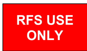
Figure 8 Example of small-bore suction connections signage
