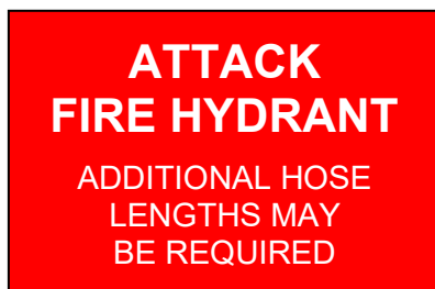
Figure 5 Example of extended coverage from external attack hydrant signage
