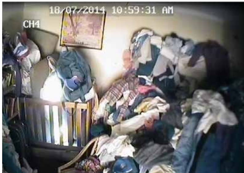
Figure 4: Ignition from lit paper placed at the bottom of material pile in cot (Test 1)
