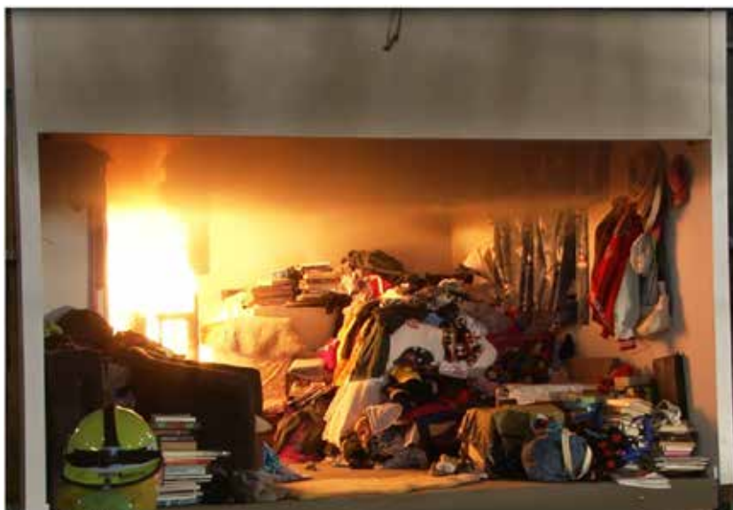
Figure 12: Early fire growth and fire spread (Test 2)
