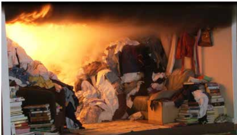
Figure 8: Early fire growth and rapid fire spread (Test 1)
