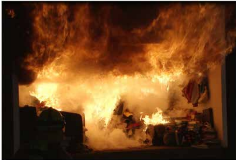
Figure 13: Fire at flashover stage – flashover was reached in 260 seconds (Test 2)
