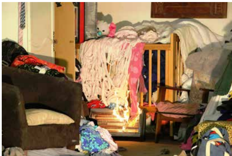
Figure 5: Ignition from radiant bar heater showing first material ignited (Test 2)
