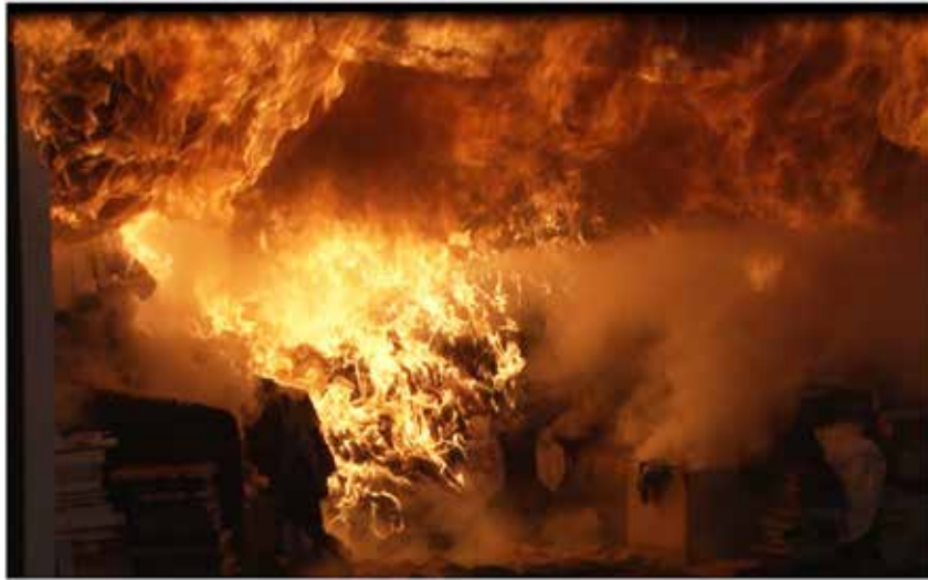
Figure 9: Fire at flashover stage – flashover was reached in 100 seconds (Test 1)
